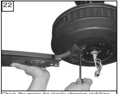
Check the motor for plastic shipping stabilizer tabs, and remove them if they are present. The screws, washers, and motor pads are preinstalled to the blade holders. Attach blade assembly to motor and tighten screws securely
